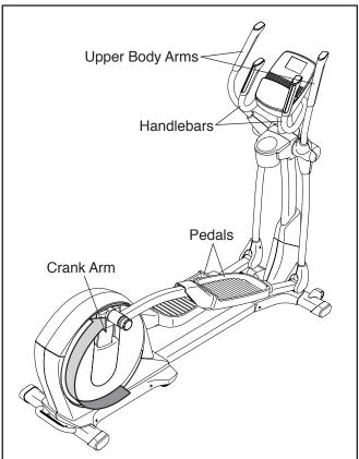
To dismount the elliptical, wait until the pedals come to a complete stop. **Note: The elliptical does not have a free wheel; the pedals will continue to move until the flywheel stops.** When the pedals are stationary, step off the highest pedal first. Then, step off the lowest pedal.
